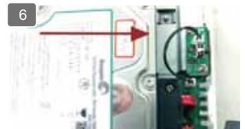
Attach the HDD to the SATA connector by sliding it toward the connector
