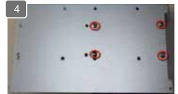
Once the tray is removed from the unit, notice there are four holes, which are used to secure the HDD.
