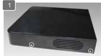
Use a screw driver to release the screws.
