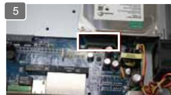
Place the HDD on the tray and secure the HDD with the screws at the bottom (as illustrated)
