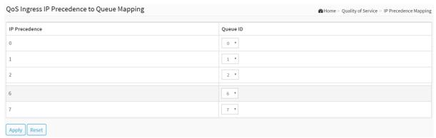
Figure 7-9: The QoS Ingress IP Precedence to Queue Mapping
