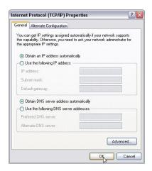
Or select "Use the following IP address" and enter the IP address, Subnet mask, Default gateway as follows:
