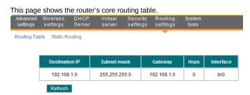
The main duty for a router is to look for a best path for every data packet, and transfer this data packet to a destination station. In order to fulfill this function, many transferring paths, i.e. routing table, are saved in the router, for choosing when needed.
