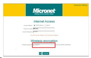
NOTE: The wireless password can only be 8 characters in length and the default is 12345678, you can modify it when necessary.
