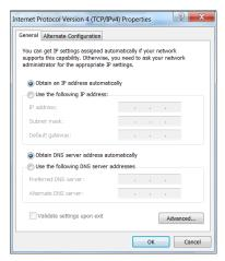
Or select "Use the following IP address" and enter the IP address, Subnet mask, Default gateway as follows:
