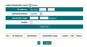
Enable Bandwidth Control: To enable or disable the internal IP bandwidth control. The default is disabled.
