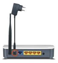
2. Please connect the LAN port of the Router to the network adapter of your computer with a cable.
